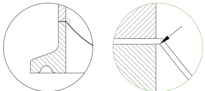
**Figure 2 – Rupture Disc foil-Carriage Intersection**
