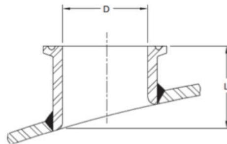
**Figure 10 - L/D for Vessel Openings**
