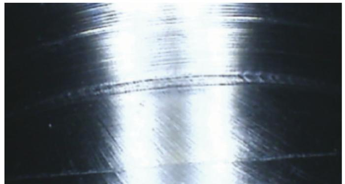
Figure 8 – Crevice View - Post Test & Rupture Disc Joining Weld (Dry) – (White lighting)
