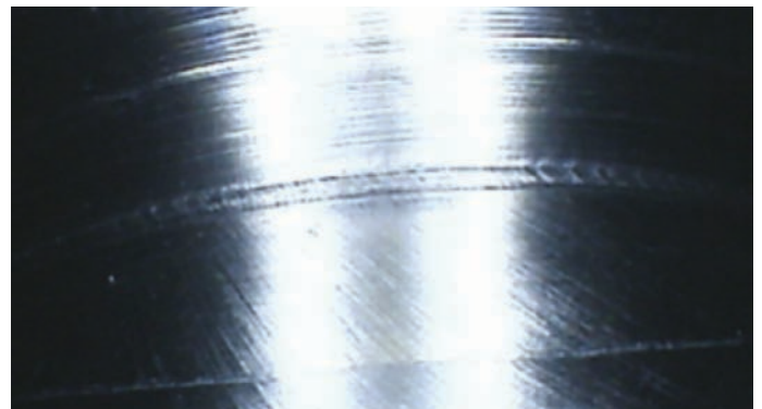
Figure 8 – Crevice View - Post Test & Rupture Disc Joining Weld (Dry) – (White lighting)
