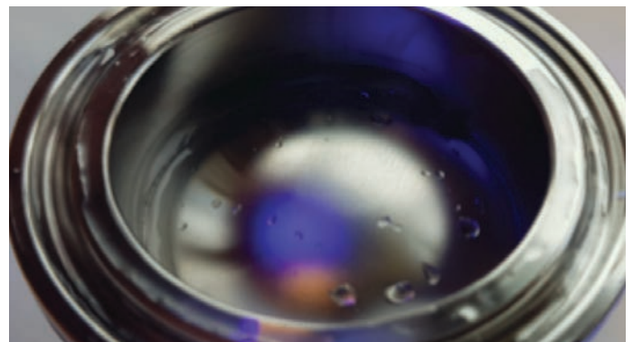
Figure 7 – Rupture Disc Carriage after Cleaning Cycle (UV lighting)
